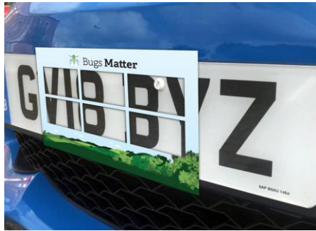
Figure 1. Photograph showing the splatometer positioned over a number plate.
